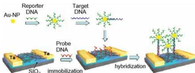
Figure I.14. 61 Schematic illustration of DNA detection enhancement by reporter DNA-AuNP conjugates.
