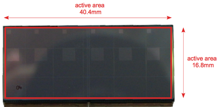
Figure 4.9.: Picture of a IBL Double Chip Sensor with the dimension of the active area.
