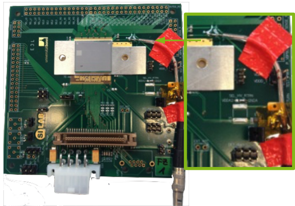
Figure 5.18.: SCC with new soldered cable for bias voltage.
