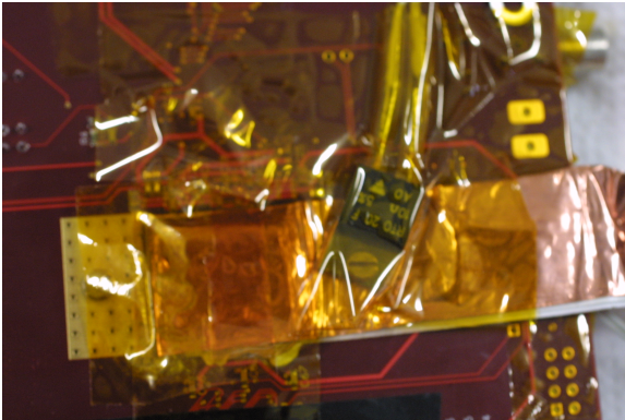
Figure 7.2.: Heating resistor mounted on the backside of LUB4.
