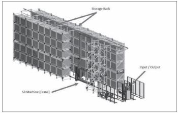
Figure 2-3: AS/RS and its components
