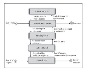
Figure 3-12: General Interface model for control levels.
