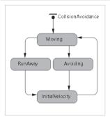
Figure 4-9: Collision Avoidance State Chart.
