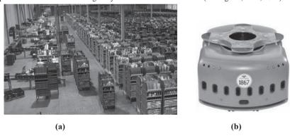
Figure 2-5: a) A Kiva warehouse implementation Flipse 2011 b) A Kiva robot Flipse 2011.
