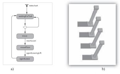
Figure 4-11: a) Left/ Right Lift State Chart, b) Screenshot of Left Lift
