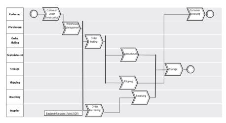
Figure 4-4: The main processes of the Cellular Transport System with their organization structure.
