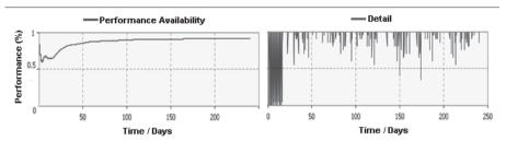
Figure 5.17: Average performance availability of shuttles calculated based on waiting time.
