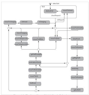
Figure 4-8: The State Chart of Multi-Shuttle Behaviour.
