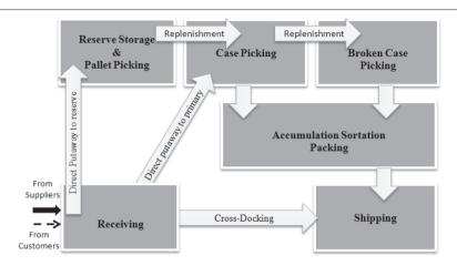
Figure 2-2: Typical warehouse functions and flows (Tompkins, et al., 2010).
