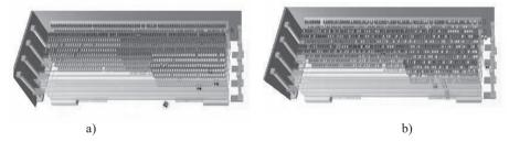
Figure 4-16: Screenshot of Class-Based Storage and Random Storage Assignment.
