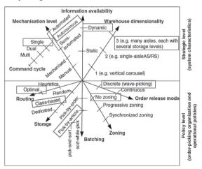
Figure 4-20: Design and Operational Parameters of the Order-picking and Storage System of the CTS based on (De Koster, et al., 2007)
