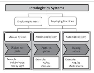
Figure 2-1: Classification of Intralogistics Systems in terms of order-picking methods (based on (De Koster, 2004)).
