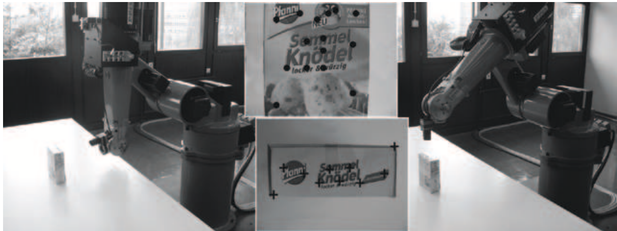
Figure 6.1: Application example for global visual servoing: start configuration (left); Disjunctive feature distribution in current and reference view (centered); Goal pose (right).
