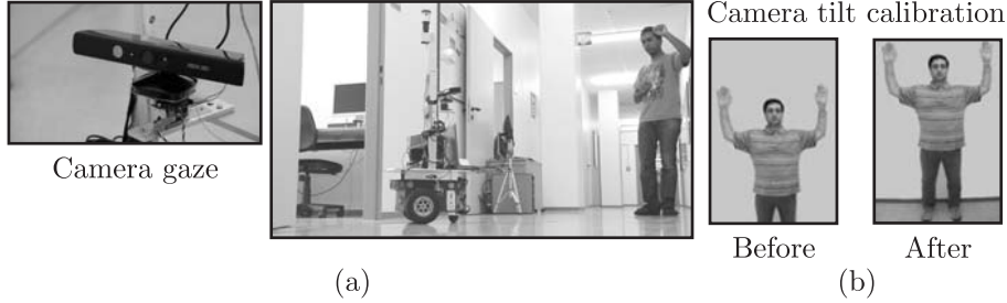
Figure 4.6.: Pan and tilt correction. (a) Camera gaze correction with a pan servo motor in action during a door traversing maneuver and (b) user image before and after tilt adjustment done during calibration.
