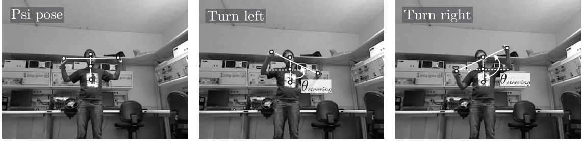
Figure 4.7.: psi pose and the steering angle poses for left and right turn
