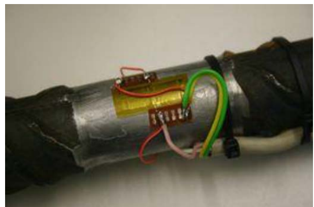
Figure 5. DMS on reinforcement bar [15]
