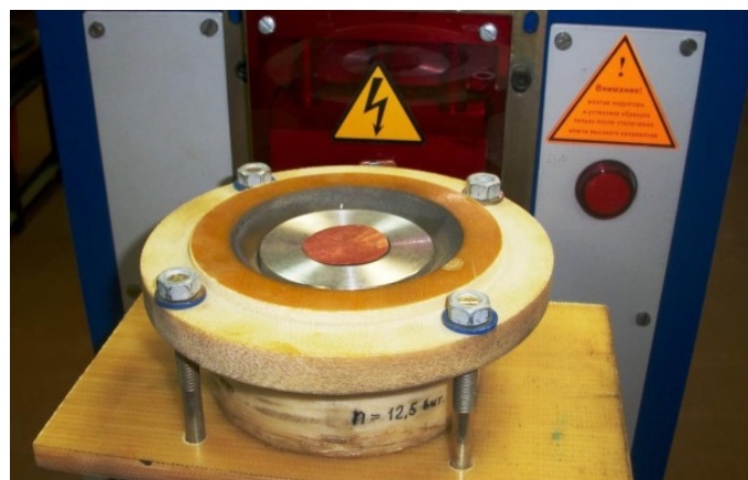
Figure 5: Inductor's arrangement for separation of metal layers.
