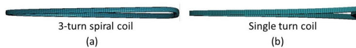
Figure 8: Predicted shapes for rings formed with the single turn and a 3-turn spiral coil
