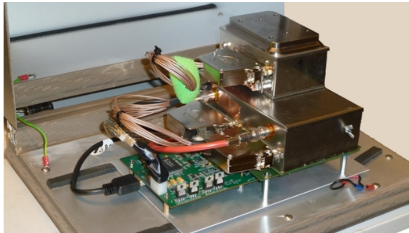
Figure 8.3: Picture of the measurement setup with IDEAS's electronics on the PCB (bottom), and the supply and connection-adapters and detectors in the metal housings on top of it. Note the extra shielded cable and the edges sealed with conductive metal tape.
