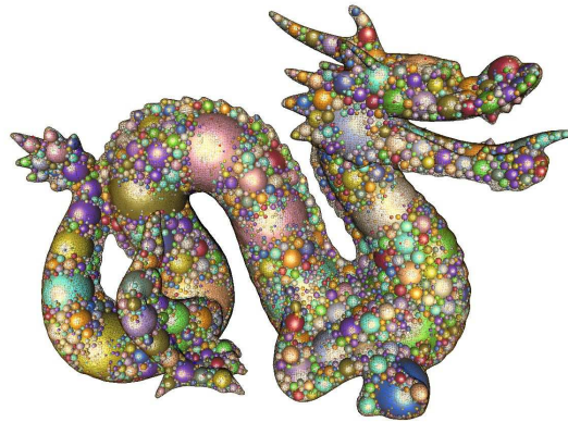
Figure 3.19: Inner Sphere Representation: the volume of the object is approximated with spheres of different size. Several inner sphere construction methods exist, the displayed version was produced by the Coll-Det software package [15, 95].
