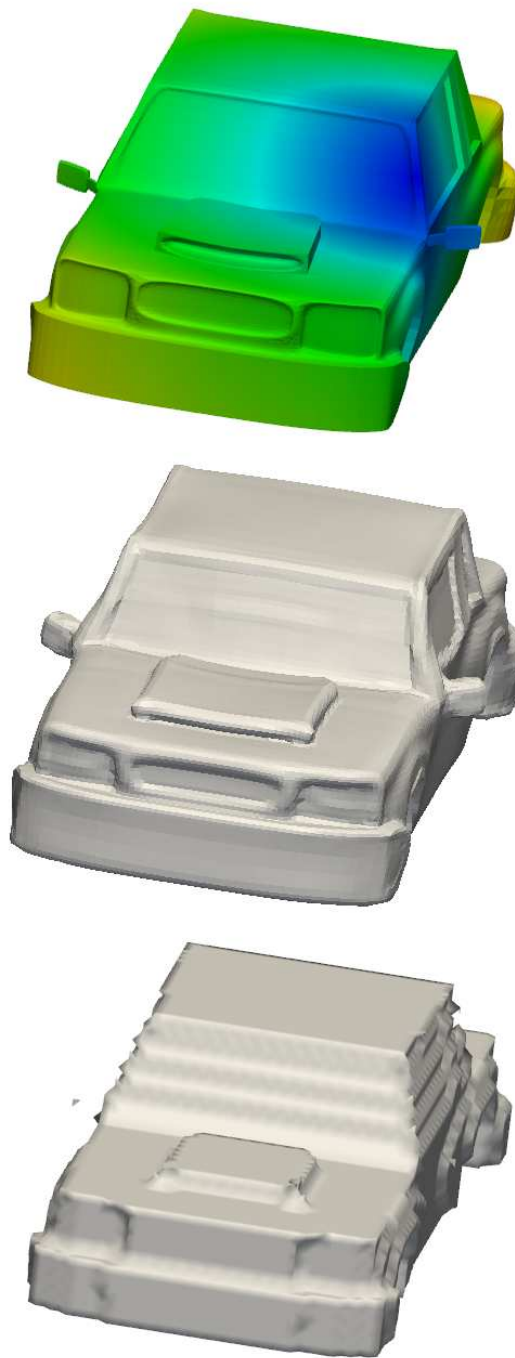
Figure 6.27: Top: original car geometry (colored with distance function), middle: mesh adaptation, bottom: no adaptation
