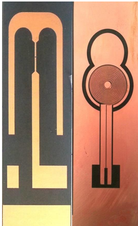
Figure 29: Picture of the printed circuit board (NMR microslot detector) after photolithography and laser ablation of the microslot (left) and circular anti-spiral heater (right).
