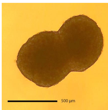
Figure 88: Microscopic image of 2 spheroids obtained with the PDMS microarray method are grown together inside the microfluidic device during the 17 hour measurements
