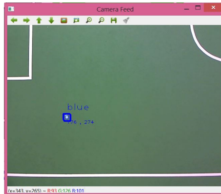
Figure 13.2: Screenshot of the developed tool while detecting a blue marker on the field.
