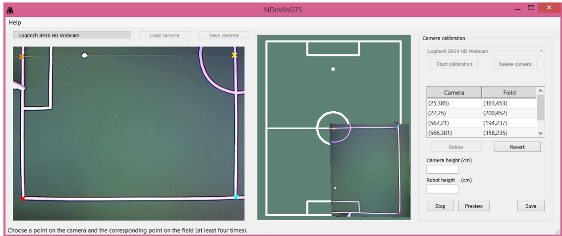
Figure 13.1: Screenshot of the developed tool after calibrating the camera. Left window shows the camera stream with the marked points, right window shows the calculated warped camera image, with the corresponding points, overlay an image of the field.
