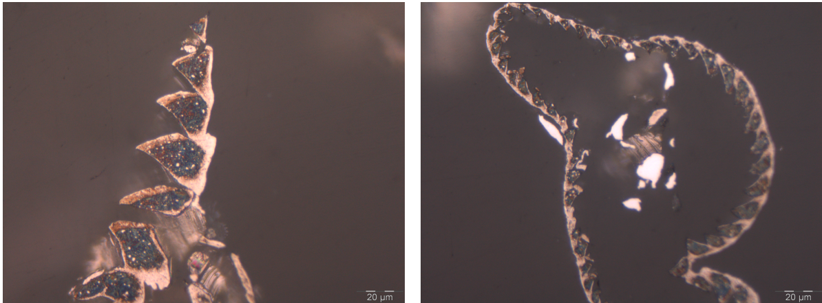
Figure 1.5: Microsections of ITG chips, cast in resin and subsequently etched. Courtesy of ISF.
