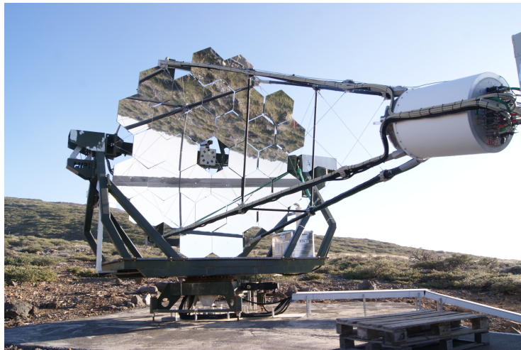
Figure 3.1: Image of the First G-APD Cherenkov Telescope in park position during the day.
