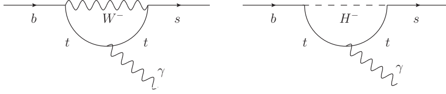
Figure 1.9: b \rightarrow s\gamma in the SM (left) and with a charged Higgs boson (right).
