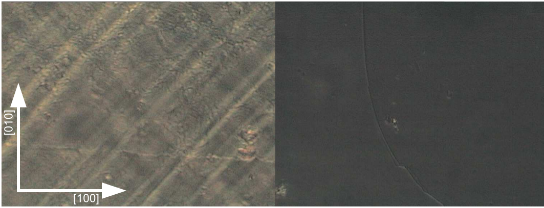
Figure 3.1: Crystal: (left side) pure NaCl, (right side) CuCl:NaCl, between crossed Nicol prisms after uniaxial pressure along [010]. The variation of light intensity in pure NaCl corresponds to birefringent bands along [110] and [1\bar{1}0] which had been written-in by the uniaxial pressure.
