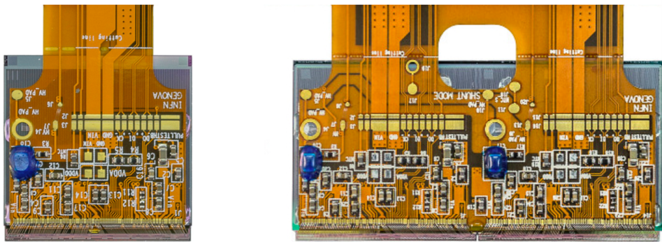
Figure 5.15: Pictures of an assembled single 3D module (left) and planar double chip module (right) [31].
