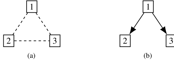
Figure 3.1: An instance of the STP where all three vertices are terminals and all edge costs are 1. (a) shows the optimum solution of the relaxed undirected cut formulation with value 1.5 by setting x_e = 0.5 for all edges e . There is no valid solution for the directed cut formulation with the same value. Instead, two arcs have to be selected, e.g., for root node 1 z_{12} = z_{13} = 1 , as depicted in (b).
