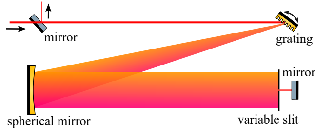
Figure 3.8: Graphical illustration of the pulse shaper. The incident light beam with a broad spectrum is diffracted by a specially designed gold grating. In combination with a gold coated spherical mirror and a slit with a small width, a narrow part of the spectrum can be separated with FWHM of \approx 1 nm.
