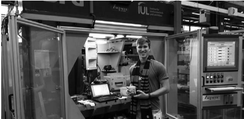
RISE exchange student Logan Gable in front of the five-axis forming press for incremental sheet-bulk metal forming operations
