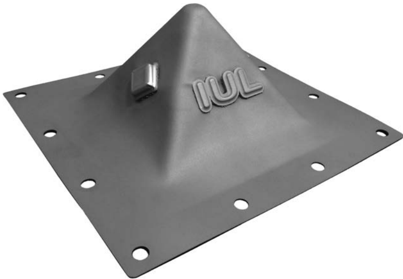
Incrementally deformed pyramid stump with additively and mechanically finished functional elements
