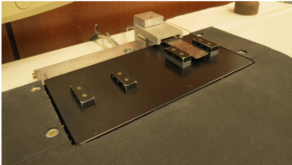
Figure 2.7: Picture of the modified tapbox. The LEDs and photodiodes of the photoelectric sensor have been raised to allow the installation of the force key.
