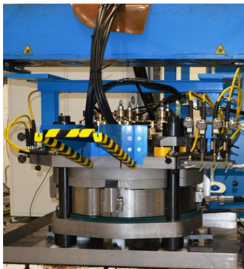
Figure 7: Set-up used at Bmax for the forming of 400 MHz and 700-800 MHz half-cells
