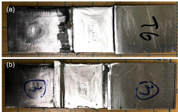
Figure 15: Spot weld of Al6061-T6 to 4130 steel as welded (a) and after lap shear test (b). Aluminum flyer failed during test for both cases of T4 and T6.
