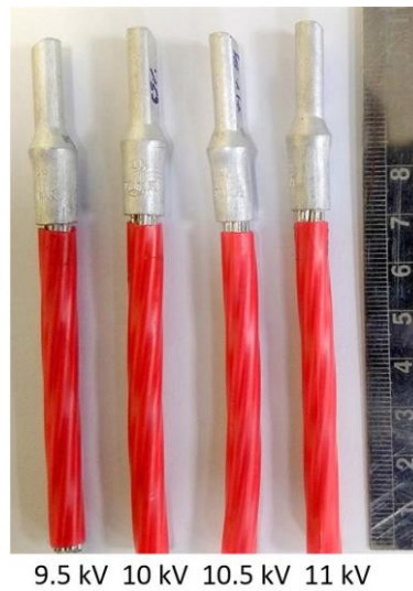
Figure 5: Samples crimped using different types of field-shaper at various discharge voltages
