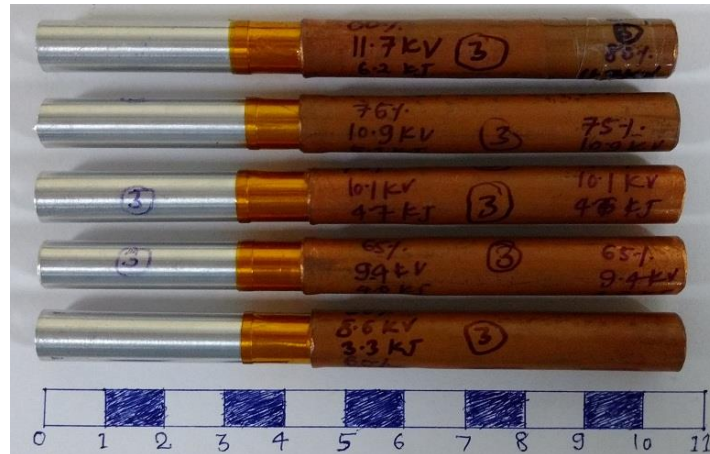
Figure 4: EMC process crimped samples
