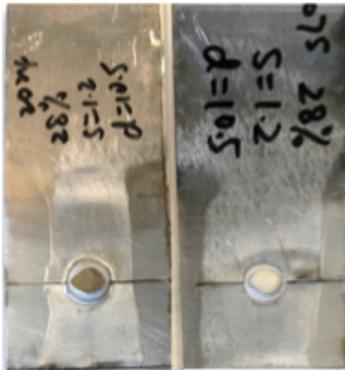
A: Pull-out failure
