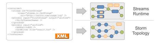
Figure 2: The XML is compiled into a data flow graph for different runtime environments. Currently the *streams* runtime is supported and a prototype for the *Storm* compiler exists.
