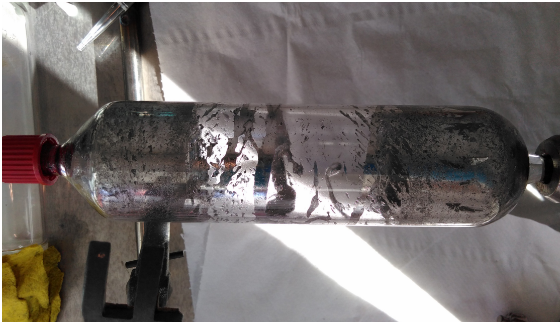
Figure 2.16.: Partially wetted reactor with 4mL of GaInSn
