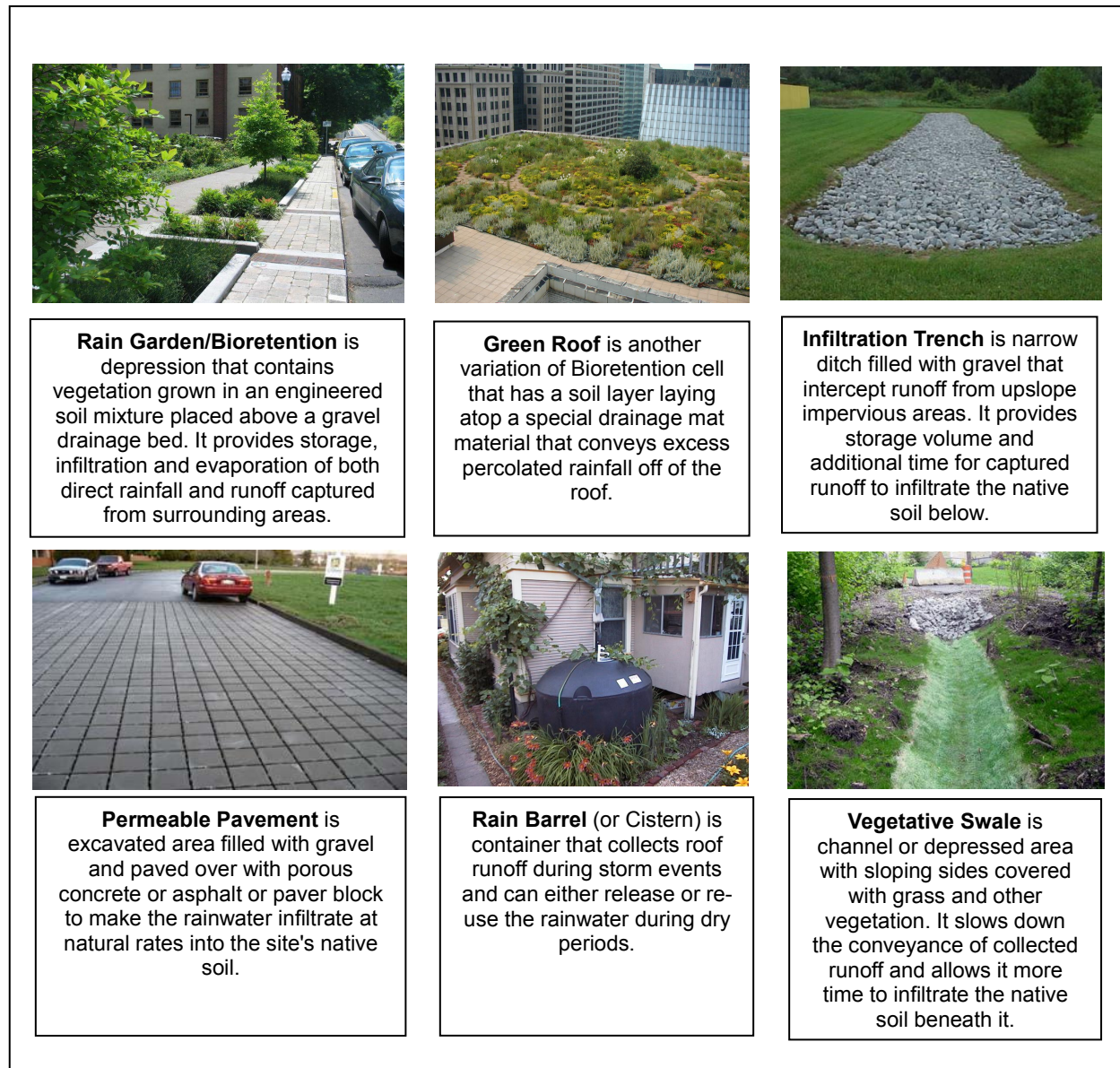
Figure 2-3: Typical LIDs ( USEPA, 2015)
