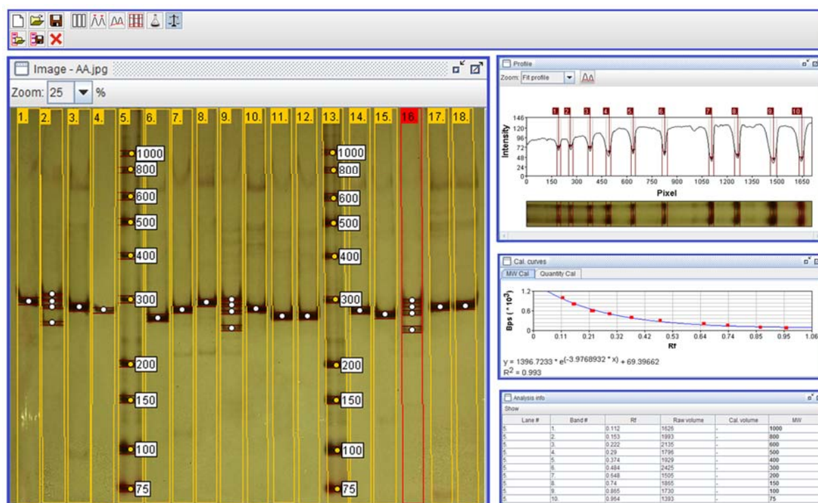
Figure 1: Genotyping of AR-CAG polymorphism by Gel Analyzer software. The genotype of the samples is determined on the polyacrylamide gel in the software, and the size of the bands is estimated by the ladder calibration.
