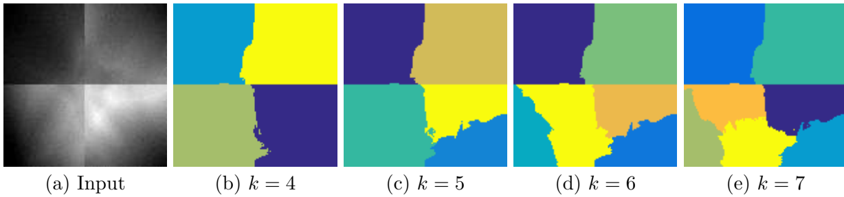
Figure 5.14. (a) Input median image of synthetic dataset. (b-e) Normalized cuts segmentation of median image, the colors code different surface segments. Reasonable results are only achieved for k \in \{4, 5\} .
