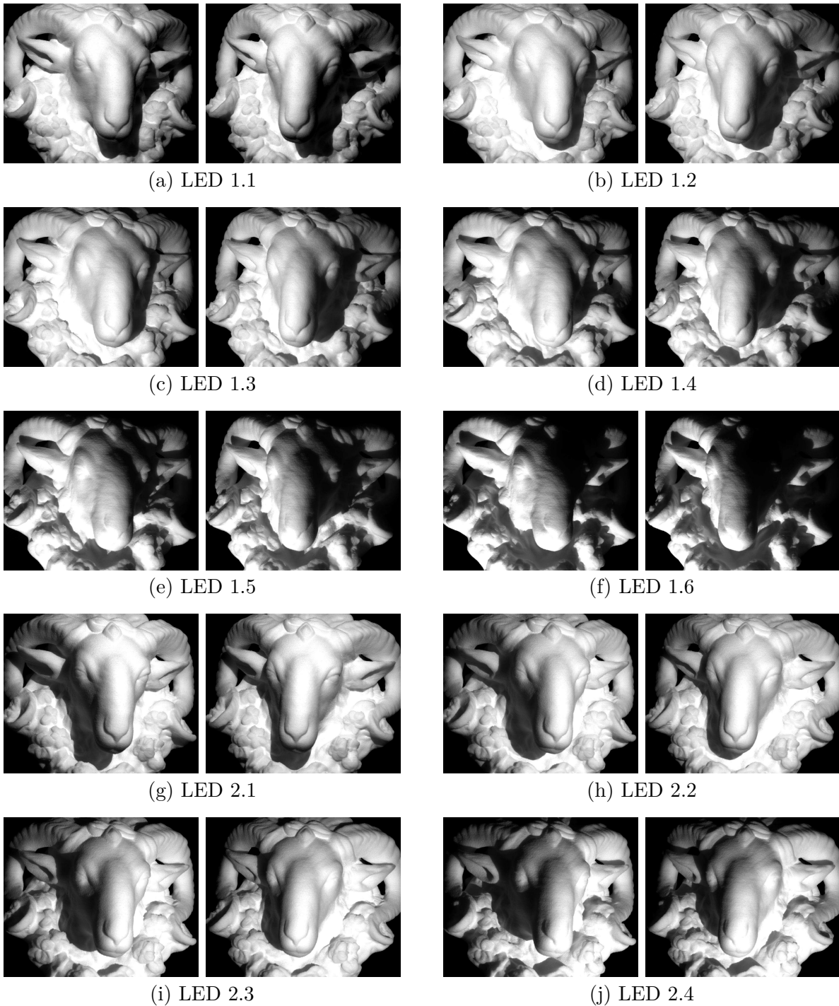
Figure A.6. Left and right stereo input images of the ram dataset used to evaluate the Stereo Fusion algorithm. Same scaling in corresponding stereo pairs.
