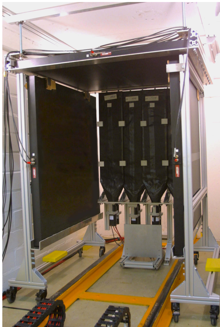
Figure 6.11.: New scintillation detectors integrated into the muon veto detector of the DLB together with the backside that is still consisting of eight scintillators with 5 mm thickness in a interlaced two-layer setup.
