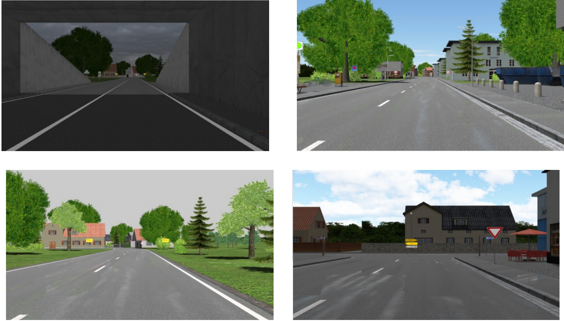
Figure 3.19: Sample images of the complex test route used as training data for the neural-network-based lane detection
