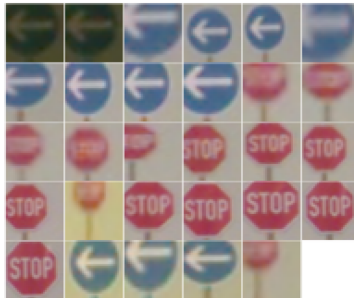
Figure 5.29: Multiple Sequences of consecutive frames with detected cropped street signs. These are the input features for the street sign classifier
