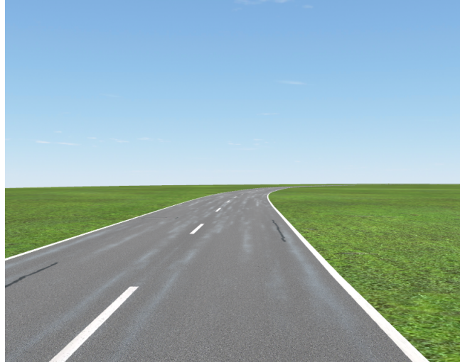
Figure 3.17: First simple track to test lane detection and steering control for lane keeping on.
