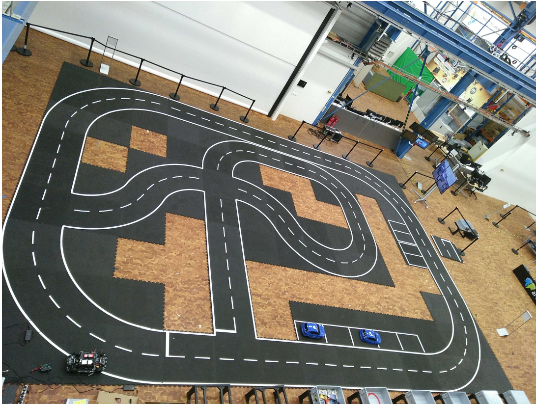
Figure 3.20: Overview of the real test route build with floor mats
