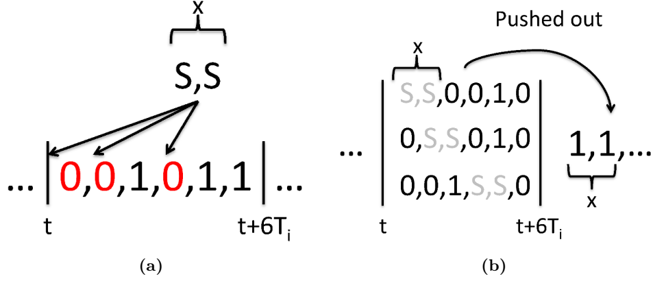
Figure 4.2: Example of successful executions in the proof of Theorem 2, in which (a) is the original jobs of \tau_i and (b) is the jobs of \tau_i after the insertion. x number of S insertions at most only push out x reliable jobs.
