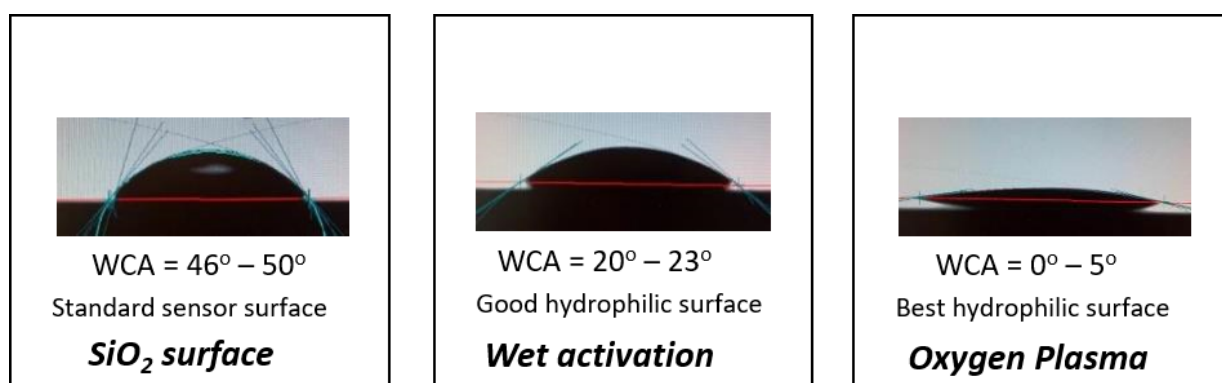
Figure 3.5: Measured water contact angle before and after wet chemical and plasma induced surface activation.
