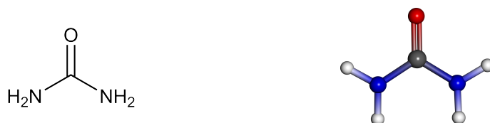
Figure 1.2.: 2D (left) and 3D (right) structure of urea. The red bead represents oxygen (O), the black bead carbon (C), the blue beads nitrogen (N) and the white beads hydrogen (H).
