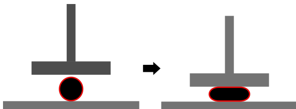
Figure 5.5.: Visualization of the capsule compression measurement. This graphic has been created by E. Zwar and has already been published in ref. [148].
