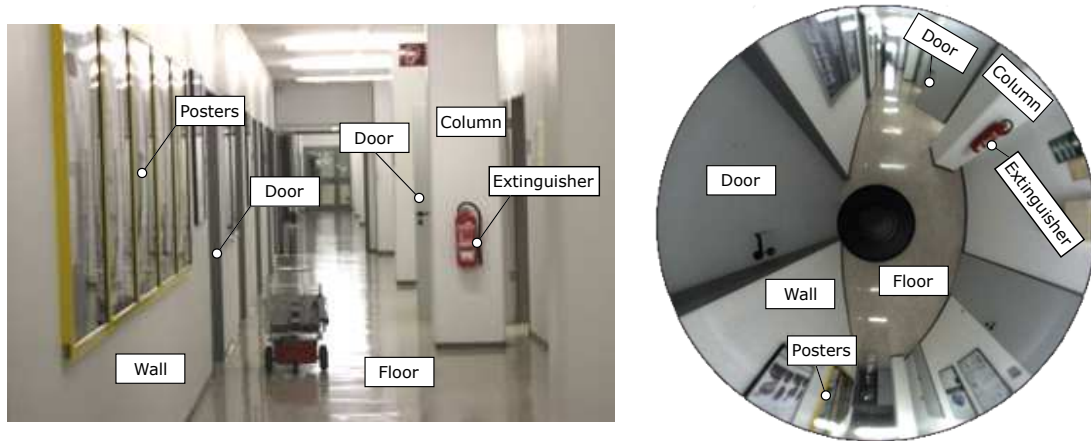
Figure 1.2: Experimental platform positioned on a scene where the omnidirectional image at the right was captured. The scene and the omnidirectional image are labeled with the same objects to show the wide field of view image formation and distortion introduced by the hyperbolic mirror
