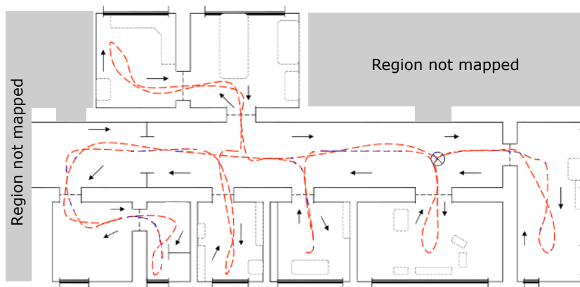
Figure 8.5: Sketch of the Freiburg floor plan (COLD Dataset). The dotted red line indicates the sequence followed by the robot while acquiring the sensor data
