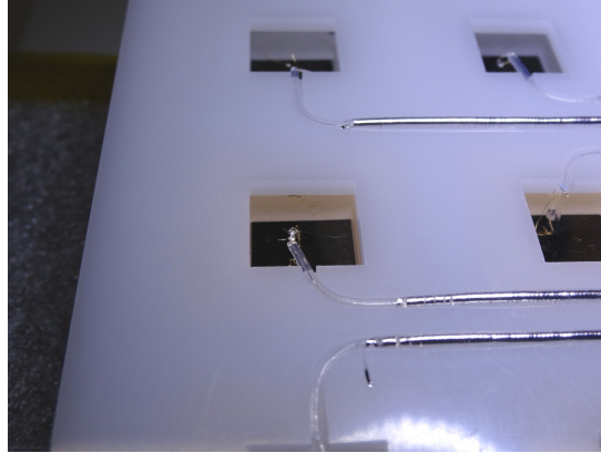
Figure 4.10: Close-up photograph of high-voltage contacts of XDEM detectors.
