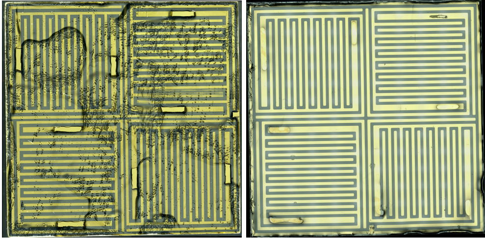
Figure 4.4: Comparison of GLYPTAL coating (left) applied by EV and epoxy coating applied by the author (right). The coating on the left seems much more in-homogeneous and small inclusions are visible in a number of spots.
