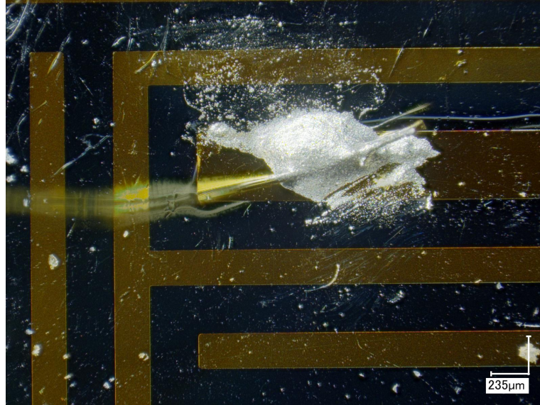
Figure 4.8: Connection of gold wire and anode of a test detector with conductive silver-based epoxy.
