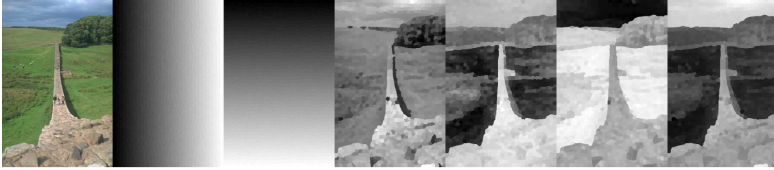
Figure 5.1: Overview of the used feature channels for an exemplar image of the training set of the BSDS500. Due to the proposed superpixel sampling the superpixel structure is visible in every channel. From left to right: image, x-position, y-position, three colour channels, and texture channel.
