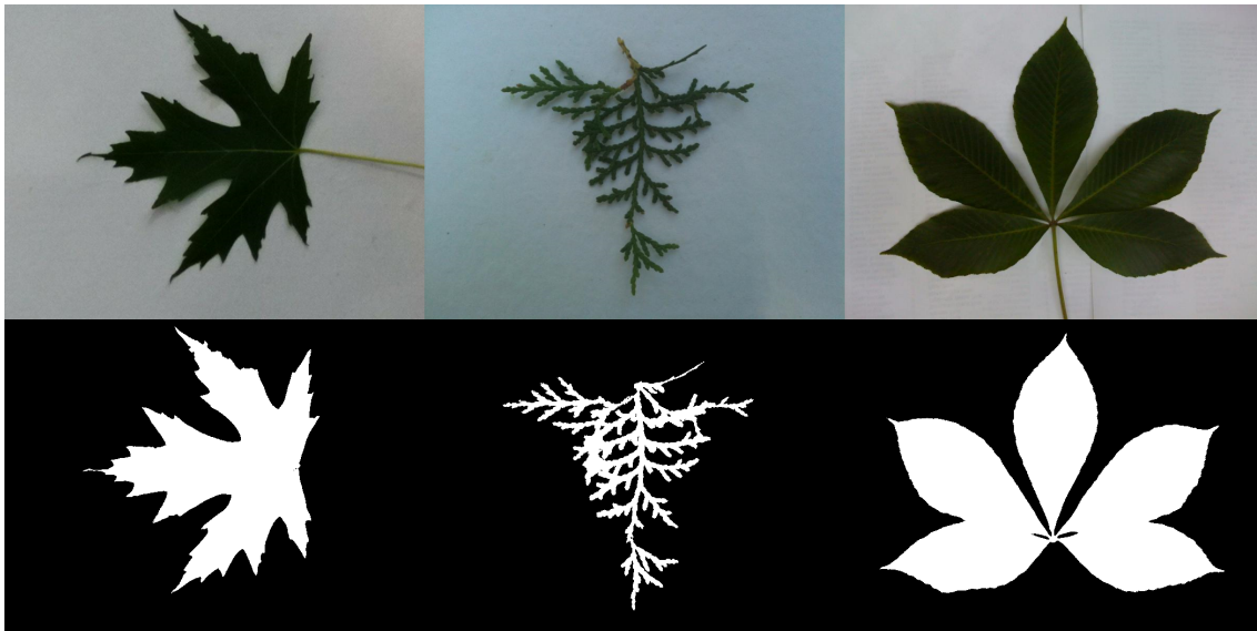
Figure 2.6: Three sample images (top row) of the LeafSnap Field data set [Kum+12]. The ground truth annotations (bottom row) are binary and the stems are intentionally excluded from the ground truth, because they do not contribute strongly to distinguishing different genera.
