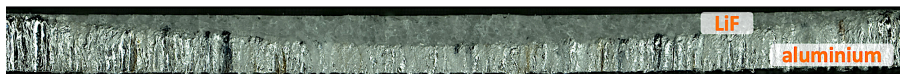
Figure 3.8: Cross-section of a neutron TL-DOS detector produced with LiF:Mg,Ti in powder configuration. The detector is cut in the middle by a laser.
