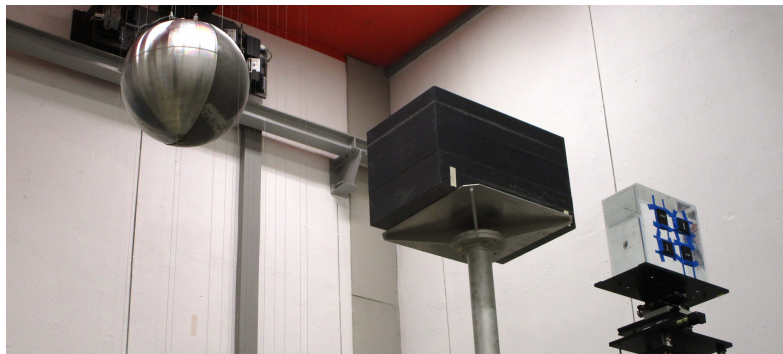
Figure 4.3: Irradiation setup for four albedo dosimeters at an ISO standard water phantom in the isotropic ^{252}\text{Cf}(\text{D}_2\text{O},\text{Cd}) + shadow object reference field at the PTB. All irradiations are performed in the low scattering room. Left: Source, middle: shadow object, right: phantom with detectors. [64]
