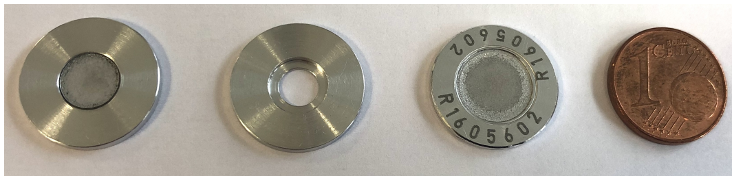
Figure 3.12: From left to right: One TL-DOS adapter in combination with a neutron detector, only an adapter for readout of small elements with the TL-DOS standard reader, standard TL-DOS whole body detector, 1 cent coin to compare all sizes.
