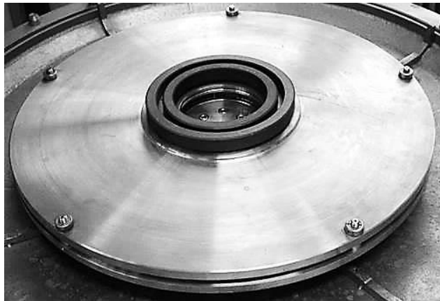
Fig. 60. RPB rotor with an outer diameter of 600 mm.
