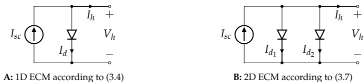
Fig. 3.5 Ideal equivalent circuits of I-V characteristics for a PV transducer.
