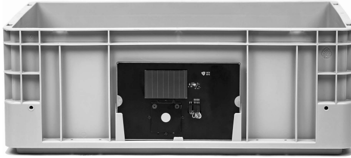
Fig. 3.15 Developed board for the measurement of IPV data, mounted on a box. This board houses probe integration sphere and sensors in addition to the IPV module.
