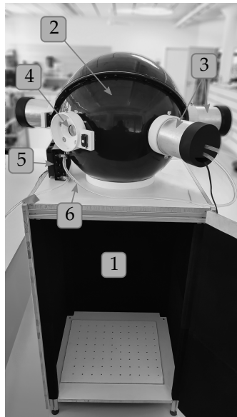
Fig. 3.17 The overall structure of the light measurement platform. 1: Interior light absorbing layer, 2: Integration sphere, 3: Input holes and light mounting device, 4: Servo controlled diaphragm, 5: Heat exchange radiator, 6: Cooling pipes
