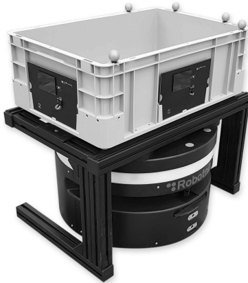
Fig. 3.34 Mobile setup for automatic measurement of environmental parameters in PhyNetLab. Two measurement boards enable measurement at different radius from the center point. Box has a set of IR reflective markers which enable exact positioning of the box at each time in PhyNetLab.
