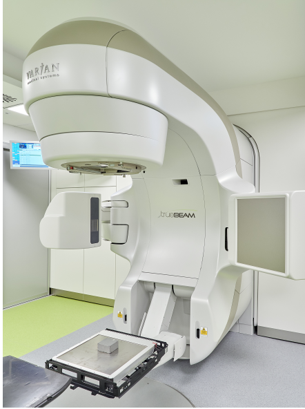
(a) Varian TrueBeam accelerator with extended PortalVision aS1200 megavoltage detector (cover removed).
