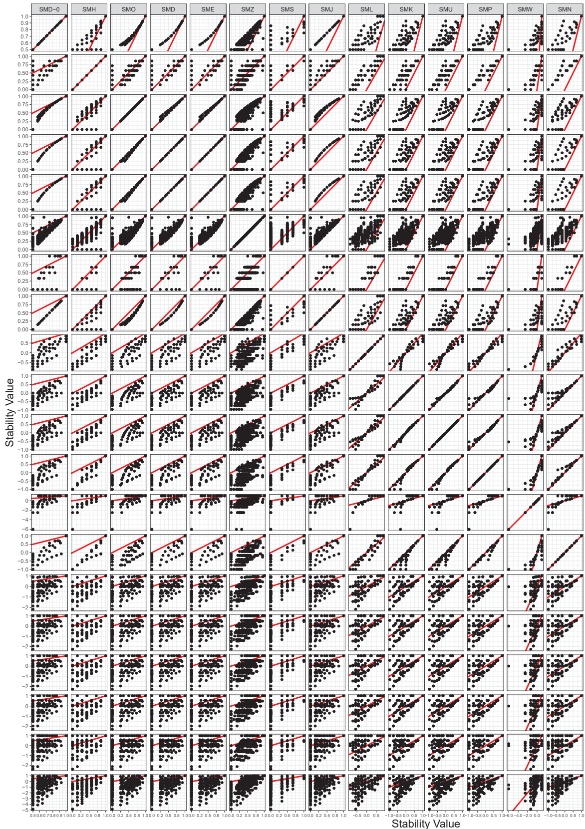
Figure 6.2: Scatter plots of the stability values obtained with the 19 stability measures for the 16 384 combinations. The red line in each plot indicates the identity. The order of the stability measures is determined by conducting a PCA with the stability measures as observations and all stability values as features, and ordering the measures by the values of the first principal component.
