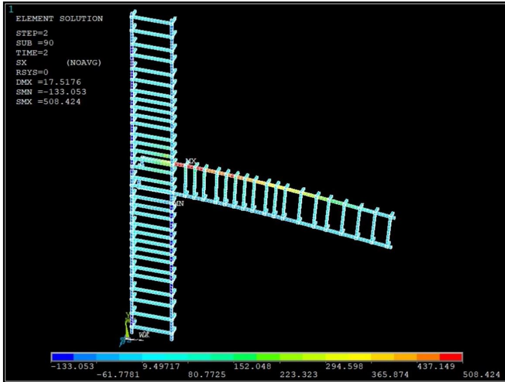
Fig 82. Axial stress of steel bars of the system with bolted SMA plate under cyclic load
