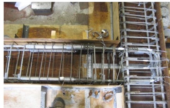
Fig 16. Experimentally investigated R.C. beam-column strengthened with SMA bars (Youssef et al., 2019)
