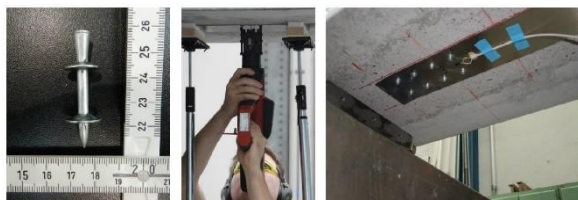
Fig 13. Reinforced concrete beam reinforced with externally bonded Fe-SMA strip (Michels et al., 2017)
