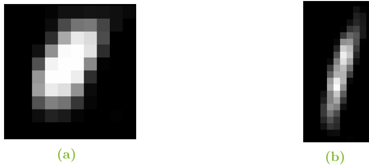
Figure 4.4: Spots of the focused laser beam. Figure 4.4a shows the spot of the ( \lambda_0 = 450 \text{ nm} , P = 1.6 \text{ W} ) diode [60] and Figure 4.4b the spot of the ( \lambda_0 = 448 \text{ nm} , P = 3.5 \text{ W} ) diode laser [52]. CCD Camera: 1/3 in S/W A1-Pro , Conrad Electronics , Germany
