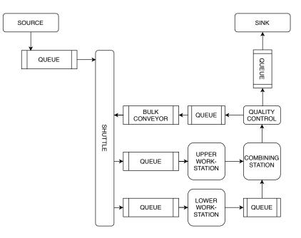
Figure 6.8: The DOSIMIS-3 simulation model.
