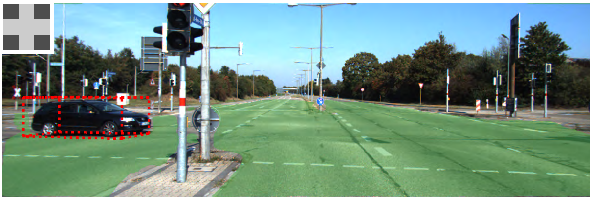
Figure 1.2: Illustration of three camera-based environment representations. Red: enclosing 3D bounding box of other present road users. Green: segmentation of the drivable road area. Top left: global context of the prevailing road topology
