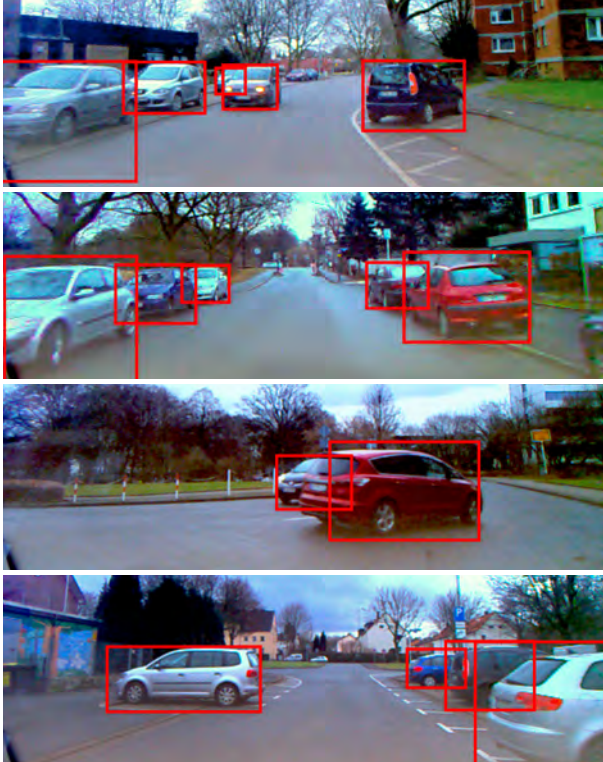
Figure 7.10.a: Example 2D detections of the Plain-SSD model on the InVerSiV test dataset.
