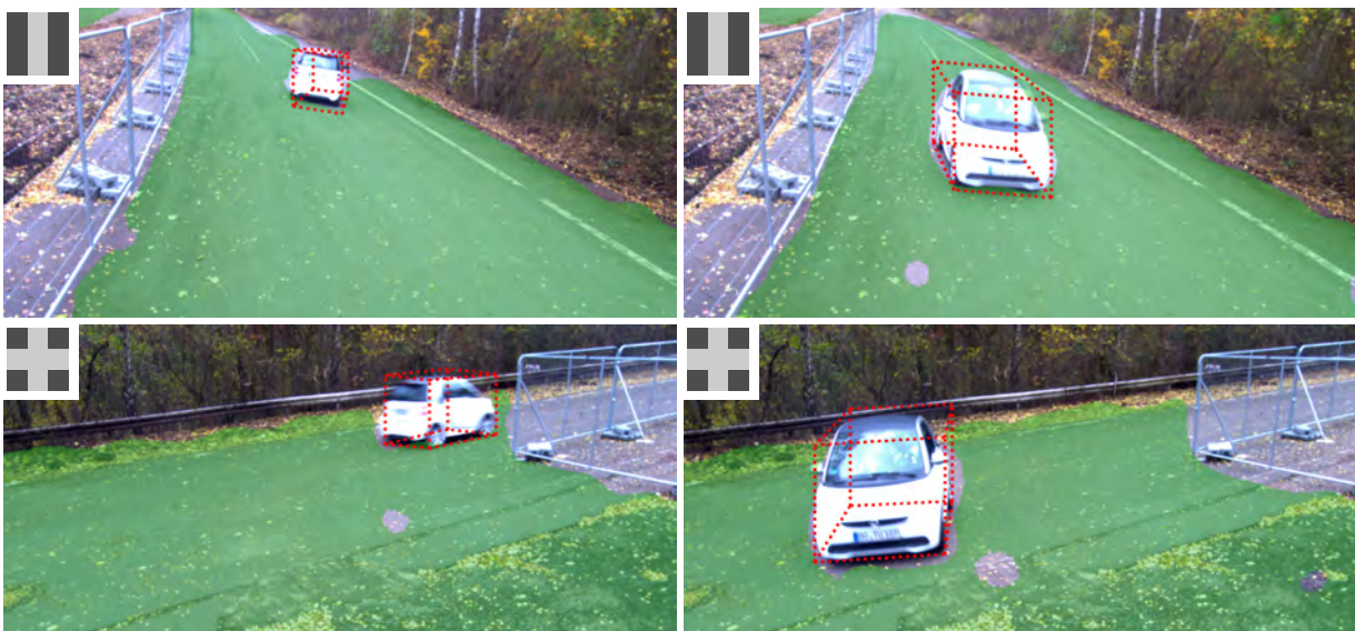
Figure 8.4: Visualization of the environment representations generated with the full multi-task model in the InVerSiV road side unit setup. Due to the altered operating conditions, the input images differ significantly from those of the used training dataset.
