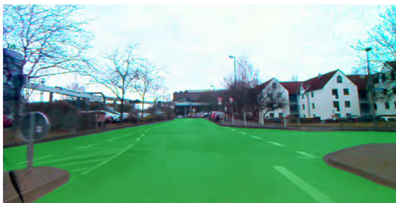
Figure 6.1: Example image recorded from the test vehicle near TU Dortmund University. The ground truth annotations of the drivable road area are highlighted in green.
