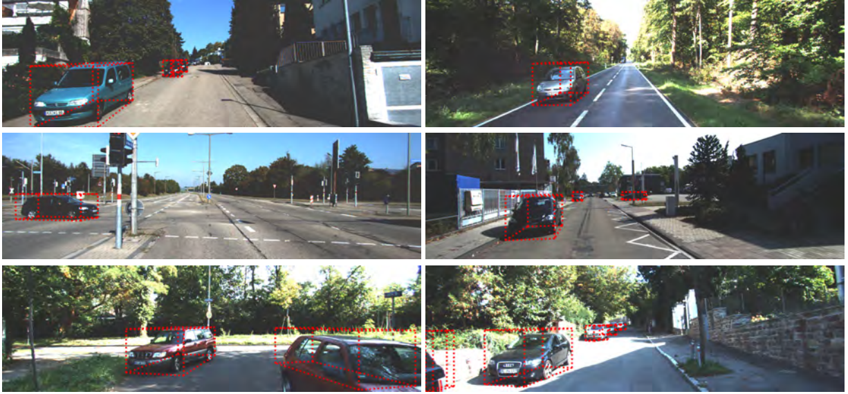
Figure 7.11: Example 3D detection boxes of the SSD-AUX model on the KITTI object validation dataset.
