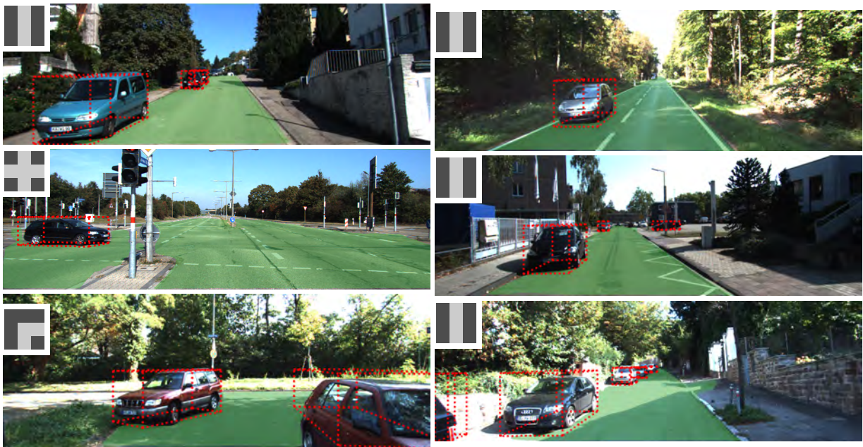
Figure 8.3: Visualization of the environment representations generated with the full multi-task CNN. The example images originate from the validation partition of the KITTI object dataset.
