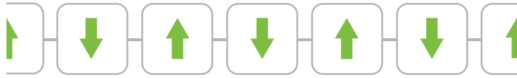
Figure 2.5: Illustration of the one-dimensional Heisenberg model in real space. The system consists of fixed spins which interact via exchange coupling with each other. No hopping processes of particles can take place.
